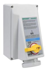
Bryant pin and sleeve mechanical interlock, rotary, enclosed, load break capable, 240 VAC, 60A, 1-phase, 2-pole, 3-wire, 6 hour pin and sleeve receptacle, 10kA SCCR, 11.9in x6.9in x8.6in housing.
