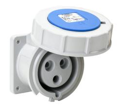
Bryant watertight single pin and sleeve receptacle, 30A, 250 VAC, 1-phase, 2-pole, 3-wire, 6 hour, IP67, nylon housing, blue.
