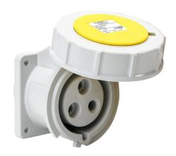
Bryant watertight single pin and sleeve receptacle, 30A, 125 VAC, 1-phase, 2-pole, 3-wire, 4 hour, IP67, nylon housing, yellow.
