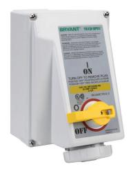
Bryant pin and sleeve mechanical interlock, rotary, enclosed, load break capable, 120 VAC, 30A, 1-phase, 2-pole, 3-wire, 4 hour pin and sleeve receptacle, 10kA SCCR, 10.1in x6.9in x7.8in housing.
