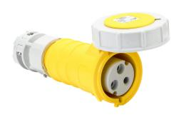
Bryant watertight pin and sleeve connector, 20A, 125 VAC, 1-phase, 2-pole, 3-wire, 4 hour, accepts cord size 0.37-0.595in, IP67, nylon housing, yellow.
