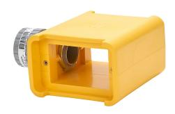
Bryant dead end portable outlet box, (1) 3/4in female NPT conduit entries, accepts cord size 0.38 - 0.5in, NEMA 1, PBT thermoplastic elastomer housing, yellow.
