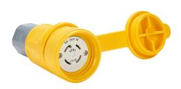
Bryant watertight locking blade connector with cap, 30A, 250 VAC, 3-phase, 3-pole, 4-wire, NEMA L15-30, accepts cord size 0.385-1.05in, UL Type 4, 4X, 6 and 6P, thermoplastic elastomer (PTE) housing, yellow.
