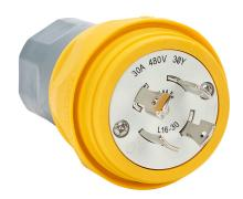
Bryant watertight locking blade plug, 30A, 480 VAC, 3-phase, 3-pole, 4-wire, NEMA L16-30, accepts cord size 0.385-1.05in, UL Type 4, 4X, 6 and 6P, thermoplastic elastomer (PTE) housing, yellow.
