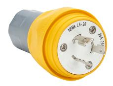
Bryant watertight locking blade plug, 20A, 250 VAC, 1-phase, 2-pole, 3-wire, NEMA L6-20, accepts cord size 0.325-0.75in, UL Type 4, 4X, 6 and 6P, thermoplastic elastomer (PTE) housing, yellow.
