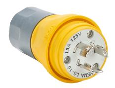
Bryant watertight locking blade plug, 15A, 125 VAC, 1-phase, 2-pole, 3-wire, NEMA L5-15, accepts cord size 0.3-0.62in, UL Type 4, 4X, 6 and 6P, thermoplastic elastomer (PTE) housing, yellow.
