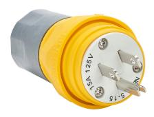
Bryant watertight straight blade plug, 15A, 125 VAC, 1-phase, 2-pole, 3-wire, NEMA 5-15, accepts cord size 0.325-0.625in, UL Type 4, 4X, 6 and 6P, thermoplastic elastomer (PTE) housing, yellow.
