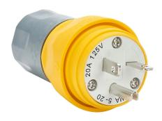
Bryant watertight straight blade plug, 20A, 125 VAC, 1-phase, 2-pole, 3-wire, NEMA 5-20, accepts cord size 0.325-0.625in, UL Type 4, 4X, 6 and 6P, thermoplastic elastomer (PTE) housing, yellow.
