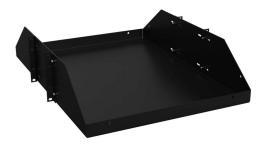
Hammond heavy duty rack shelf, 3U, 19in rack width, 24in depth, 550lb capacity, carbon steel, black, powder coat finish.
