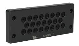
Bimed BRM series cable entry system frame, nylon frame, 24mm, black, (23) 4-8.5mm opening(s), IP65.
