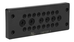
Bimed BRM series cable entry system frame, nylon frame, 24mm, black, (16) 3-6.5mm, (4) 5-9.2mm and (2) 8-12.5mm opening(s), IP65.
