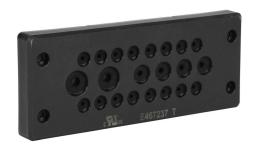
Bimed BRM series cable entry system frame, nylon frame, 24-pin frame, black, (16) 3-6.5mm, (4) 5-9.2mm and (2) 8-12.5mm opening(s), UL Type 12, 13 and 4X, IP65.
