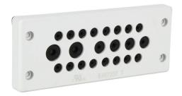
Bimed BRM series cable entry system frame, nylon frame, 24-pin frame, gray, (16) 3-6.5mm, (4) 5-9.2mm and (2) 8-12.5mm opening(s), UL Type 12, 13 and 4X, IP65.
