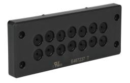
Bimed BRM series cable entry system frame, nylon frame, 24-pin frame, black, (14) 5-11mm opening(s), UL Type 12, 13 and 4X, IP65.
