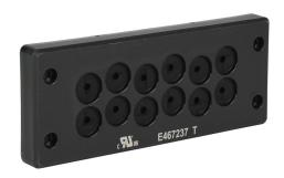
Bimed BRM series cable entry system frame, nylon frame, 24mm, black, (12) 4-13mm opening(s), IP65.
