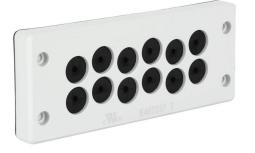
Bimed BRM series cable entry system frame, nylon frame, 24-pin frame, gray, (12) 4-13mm opening(s), UL Type 12, 13 and 4X, IP65.
