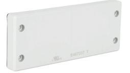
Bimed BRM series cable entry system frame, nylon frame, 24-pin frame, gray, blank opening(s), UL Type 12, 13 and 4X, IP65.
