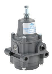
NITRA precision pneumatic regulator, 1/4in female NPT inlet(s), 1/4in female NPT outlet(s), 0-60 psi adjustable range.
