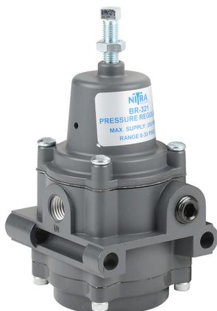
NITRA precision pneumatic regulator, 1/4in female NPT inlet(s), 1/4in female NPT outlet(s), 0-30 psi adjustable range.
