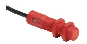
IDEM Z-Range safety switch set, non-contact uniquely coded RFID, (2) OSSD safety output(s), (1) status monitoring output(s), polyester housing, 18mm diameter x 73mm body, 8-pin M12 quick-disconnect, 9.8in/250mm cable length.
