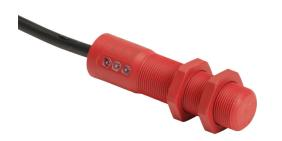
IDEM Z-Range safety switch set, non-contact uniquely coded RFID, (2) OSSD safety output(s), (1) status monitoring output(s), polyester housing, 18mm diameter x 73mm body, pigtail, 32.8ft/10m cable length.
