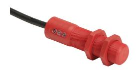
IDEM Z-Range safety switch set, non-contact master coded RFID, (2) OSSD safety output(s), (1) status monitoring output(s), polyester housing, 18mm diameter x 73mm body, pigtail, 16.4ft/5m cable length.
