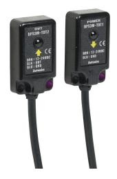
Autonics photoelectric sensor, rectangular, polycarbonate housing, through-beam pair, infrared, 0-3m sensing distance, 10.8-26.4 VDC operating voltage, dark-on, NPN, 3-wire, pigtail.
