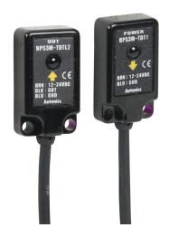
Autonics photoelectric sensor, rectangular, polycarbonate housing, through-beam pair, infrared, 0-3m sensing distance, 10.8-26.4 VDC operating voltage, light-on, NPN, 3-wire, pigtail.
