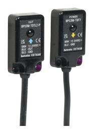
Autonics photoelectric sensor, rectangular, polycarbonate housing, through-beam pair, infrared, 0-3m sensing distance, 10.8-26.4 VDC operating voltage, light-on, PNP, 3-wire, pigtail.
