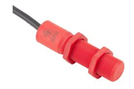
IDEM safety switch set, non-contact magnetic, (2) N.C. safety output(s), (1) N.O. monitoring output(s), polyester housing, 18mm diameter x 75mm body, 8-pin M12 quick-disconnect, 9.8in/250mm cable length.
