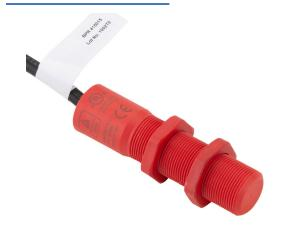
IDEM safety switch set, non-contact magnetic, (2) N.C. safety output(s), (1) N.O. monitoring output(s), polyester housing, 18mm diameter x 75mm body, pigtail, 32.8ft/10m cable length.
