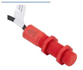
IDEM safety switch set, non-contact magnetic, (2) N.C. safety output(s), (1) N.O. monitoring output(s), polyester housing, 18mm diameter x 75mm body, pigtail, 16.4ft/5m cable length.
