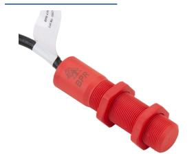
IDEM safety switch set, non-contact magnetic, (2) N.C. safety output(s), (1) N.O. monitoring output(s), polyester housing, 18mm diameter x 75mm body, pigtail, 16.4ft/5m cable length.
