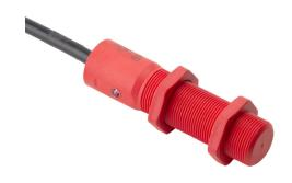
IDEM safety switch set, non-contact uniquely coded RFID, (2) N.C. safety output(s), (1) N.O. monitoring output(s), polyester housing, 18mm diameter x 75mm body, 8-pin M12 quick-disconnect, 9.8in/250mm cable length.
