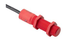
IDEM safety switch set, non-contact uniquely coded RFID, (2) N.C. safety output(s), (1) N.O. monitoring output(s), polyester housing, 18mm diameter x 75mm body, 8-pin M12 quick-disconnect, 9.8in/250mm cable length.
