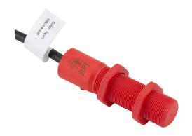
IDEM safety switch set, non-contact master coded RFID, (2) N.C. safety output(s), (1) N.O. monitoring output(s), polyester housing, 18mm diameter x 75mm body, 8-pin M12 quick-disconnect, 9.8in/250mm cable length.
