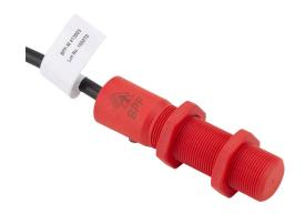
IDEM safety switch set, non-contact master coded RFID, (2) N.C. safety output(s), (1) N.O. monitoring output(s), polyester housing, 18mm diameter x 75mm body, 8-pin M12 quick-disconnect, 9.8in/250mm cable length.
