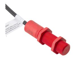
IDEM safety switch set, non-contact master coded RFID, (2) N.C. safety output(s), (1) N.O. monitoring output(s), polyester housing, 18mm diameter x 75mm body, pigtail, 32.8ft/10m cable length.
