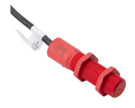
IDEM safety switch set, non-contact master coded RFID, (2) N.C. safety output(s), (1) N.O. monitoring output(s), polyester housing, 18mm diameter x 75mm body, pigtail, 16.4ft/5m cable length.
