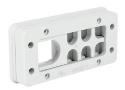
Bimed BPA series cable entry system frame, nylon frame, nylon grommet block, 24-pin frame, gray, (6) small and (1) large opening(s), UL Type 12, 13 and 4X, IP66. Requires (6) Bimed BPA series small grommets and (1) large grommets.
