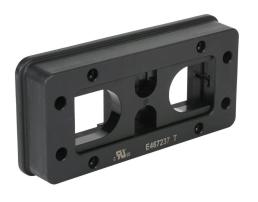
Bimed BPA series cable entry system frame, nylon frame, nylon grommet block, 24-pin frame, black, (2) small and (2) large opening(s), UL Type 12, 13 and 4X, IP66. Requires (2) Bimed BPA series small grommets and (2) large grommets.
