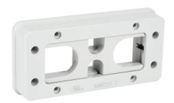
Bimed BPA series cable entry system frame, nylon frame, nylon grommet block, 24mm, gray, (2) small and (2) large opening(s), IP66. Requires (2) Bimed BPA series small grommets and (2) large grommets.
