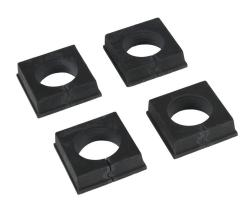
Bimed BPA series large grommet, 1 opening(s), chloroprene, black, accepts 27.5-29.5mm diameter cable, UL Type 12, 13 and 14X. Package of 4. For use with Bimed BPA series cable entry system frame.
