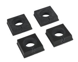
Bimed BPA series general purpose grommet, 1 opening(s), chloroprene, large, black, accepts 21.5 to 23.5mm diameter cable, IP66. Package of 4. For use with Bimed BPA series cable entry system frame.
