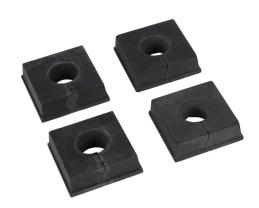
Bimed BPA series general purpose grommet, 1 opening(s), chloroprene, large, black, accepts 17.5 to 19.5mm diameter cable, IP66. Package of 4. For use with Bimed BPA series cable entry system frame.
