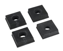
Bimed BPA series large grommet, 1 opening(s), chloroprene, black, accepts 17.5-19.5mm diameter cable, UL Type 12, 13 and 14X. Package of 4. For use with Bimed BPA series cable entry system frame.
