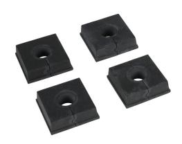
Bimed BPA series large grommet, 1 opening(s), chloroprene, black, accepts 15.5-17.5mm diameter cable, UL Type 12, 13 and 14X. Package of 4. For use with Bimed BPA series cable entry system frame.
