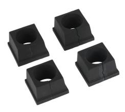
Bimed BPA series small grommet, 1 opening(s), chloroprene, black, accepts 13.5-15.5mm diameter cable, UL Type 12, 13 and 14X. Package of 4. For use with Bimed BPA series cable entry system frame.
