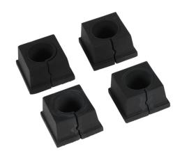
Bimed BPA series general purpose grommet, 1 opening(s), chloroprene, small, black, accepts 11.5 to 13.5mm diameter cable, IP66. Package of 4. For use with Bimed BPA series cable entry system frame.
