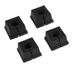
Bimed BPA series small grommet, 1 opening(s), chloroprene, black, accepts 9.5-11.5mm diameter cable, UL Type 12, 13 and 14X. Package of 4. For use with Bimed BPA series cable entry system frame.
