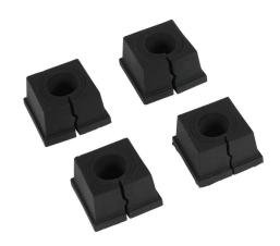
Bimed BPA series general purpose grommet, 1 opening(s), chloroprene, small, black, accepts 9.5 to 11.5mm diameter cable, IP66. Package of 4. For use with Bimed BPA series cable entry system frame.
