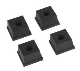
Bimed BPA series small grommet, 1 opening(s), chloroprene, black, accepts 7.5-9.5mm diameter cable, UL Type 12, 13 and 14X. Package of 4. For use with Bimed BPA series cable entry system frame.
