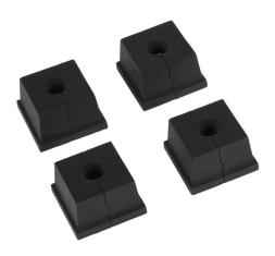
Bimed BPA series small grommet, 1 opening(s), chloroprene, black, accepts 5.5-7.5mm diameter cable, UL Type 12, 13 and 14X. Package of 4. For use with Bimed BPA series cable entry system frame.
