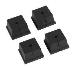
Bimed BPA series small grommet, 1 opening(s), chloroprene, black, accepts 3.5-5.5mm diameter cable, UL Type 12, 13 and 14X. Package of 4. For use with Bimed BPA series cable entry system frame.
