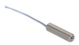
Metrol limit switch, precision touch, 5mm diameter, threaded, 0.5mm pitch, 20mm length, 3mm head, tungsten carbide, ball plunger, 1N contact force, (1) N.O. contact(s), 1.6ft/0.5m cable length, core wire.
