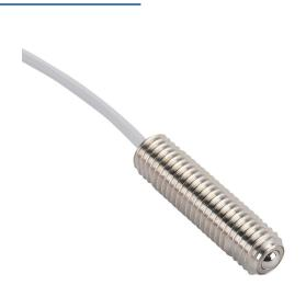
Metrol limit switch, precision touch, 10mm diameter, threaded, 1.5mm pitch, 33mm length, 5mm head, stainless steel, ball plunger, 15-20N contact force, (1) N.O. contact(s), 6.5ft/2m cable length, pigtail.
