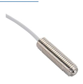
Metrol limit switch, precision touch, 10mm diameter, threaded, 1.5mm pitch, 33mm length, 5mm head, stainless steel, ball plunger, 10-20N contact force, N.O. contact(s), 6.5ft/2m cable length, pigtail.
